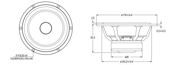
The W18E001 is a 6,5" cone driver developed for use as a high fidelity Woofer or Woofer/Midrange unit. The extremely stiff, yet light cone and the acoustically transparent basket give tremendous bass precision and midrange detail.
